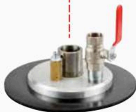
P/N 11/34 Follower plate ø 310 mm with NBR seal ring and suction tube adaptor ø 45 mm (for drum with internal ø from 260 to 310 mm).
