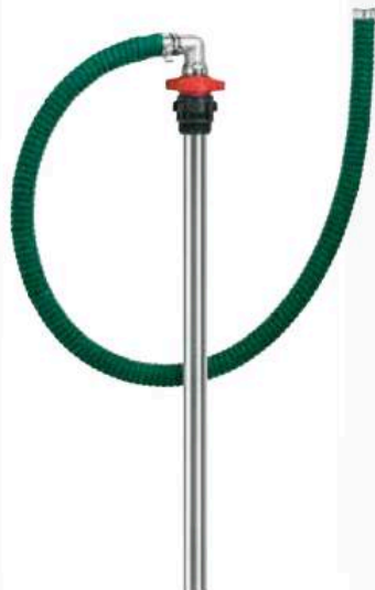
P/N 33577 AISI 304 stainless steel rigid suction tube kit \varnothing 34 mm - length 940 mm.
