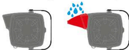
IP64 without protection cap IP65 with protection cap
