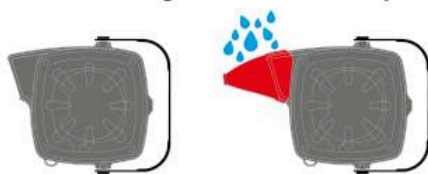
IP64 without protection cap IP65 with protection cap
